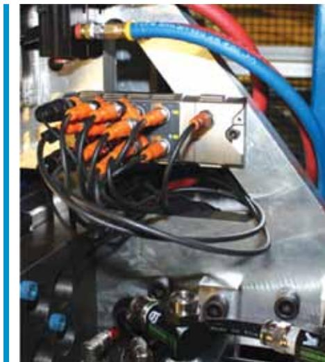
Figura 8. E/S de sensores discretos *poke-yoke*
